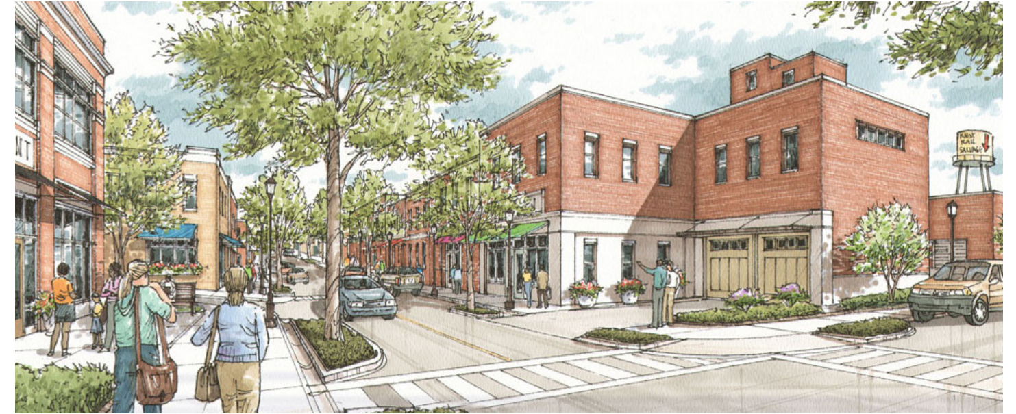
Narrowing of intersections for traffic calming and safer crosswalks
